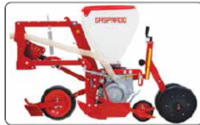
Shallow seeding furrow coulter features double rubber wheels and two rubber wheels and one smaller seed press wheel mounted behind the spike
