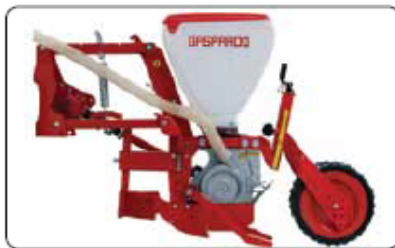
Seed boot coulter for thoroughly prepared soil.
