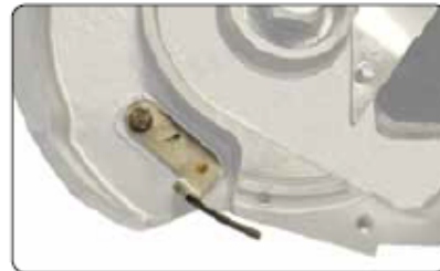
Seed expulsion unit for sugarbeet version
